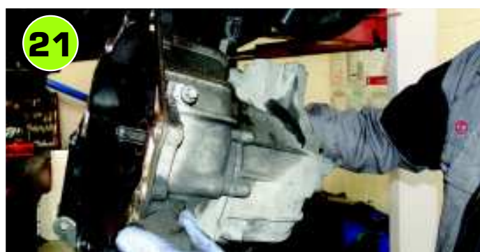
Here the gearbox is being supported on a jack with a special frame. If the cup of a trolley jack is carefully-placed it should perform the same function, ideally with two pairs of hands supporting it.
