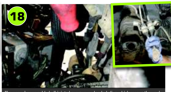
The gear change cable ball-joints have sprung-loaded clips which means they only need careful levering to remove. The bracket retaining the end of the cable is held by two bolts.
