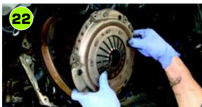
The clutch cover is loosened evenly and removed. Flywheel bolts are tight and may need a tap with a hammer on the end of the spanner to get them loose.
