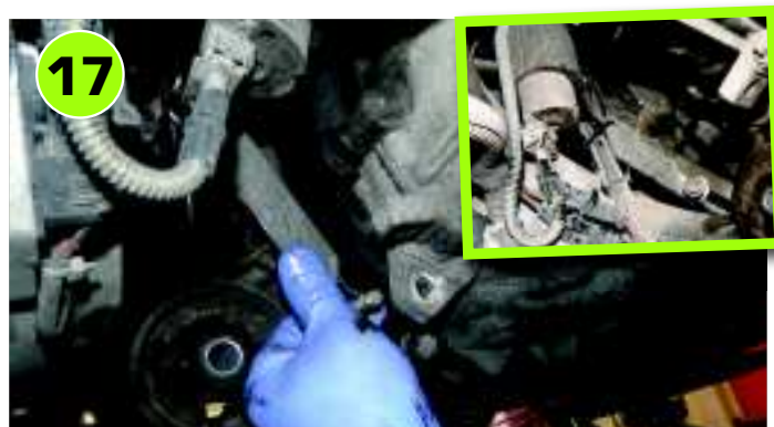
After detaching the auxiliary water pump bracket, it's recommended that it's fastened out of the way with a tie wrap to the fan housing (see inset).
