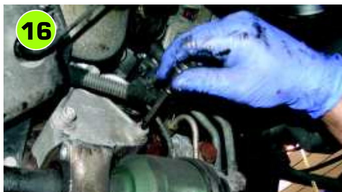
The jack shaft can be pulled from the diff after removing the three bolts from the bearing cap to loosen it off before releasing the bearing bracket.
