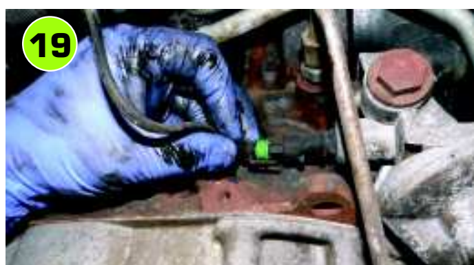
As with all wiring around the engine bed, it's best to disconnect the oil pressure sensor plug and tuck it out of the way before removing the driveshaft.
