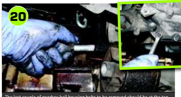
The last couple of gearbox bell housing bolts to be removed should be at the top. Some of the bolts face towards the gearbox and screw into the housing on the engine/sump side.
