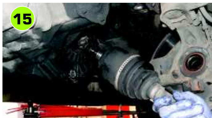
The CV joint is retained by an expansion clip on its splined shaft and only needs a strong flat-ended bar to lever it out.
