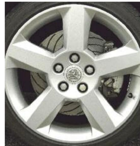
The 17in wheels (left) are from an SRi Turbo and they conceal huge 308mm Courtenay Sport discs at the front; interior (below left) is largely standard bar some tasty Irmischer detailing
