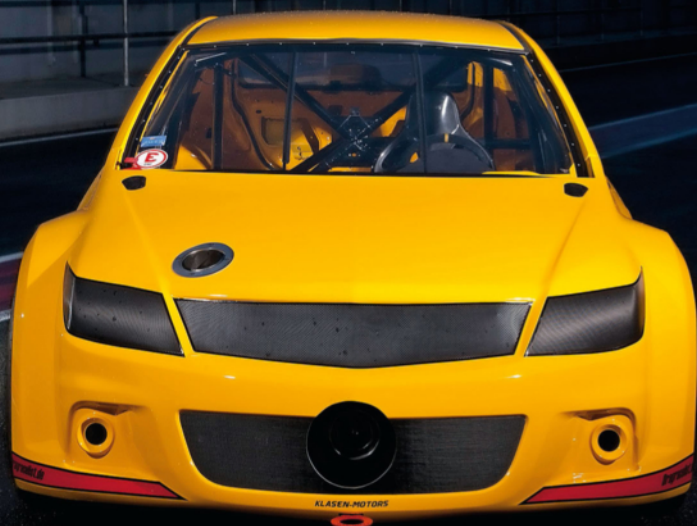
Front is dominated by the turbo and exhaust that exits the bonnet
